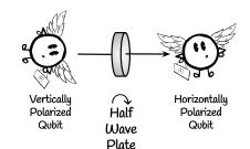
Rotates polarization of linearly polarized light
